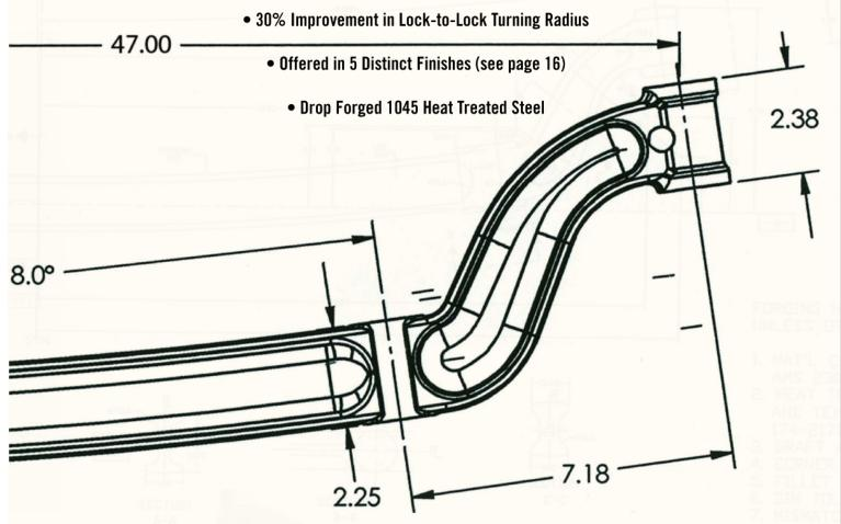
SO-CAL Speed Shop is proud to announce the addition of this forged steel I-beam axle to its New Traditionalist™ product line. SO-CAL's engineering staff spent the better part of three years refining a design that takes into account the idiosyncrasies of a reproduction part that must first work with original '37- '48 Ford spindles. The axle does that and more. It defines the quality and attention to detail customers have come to expect from SO-CAL Speed Shop.
