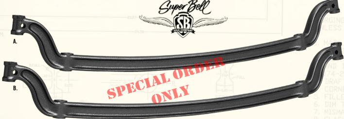
Super Bell I-beam Front Axle: The Super Bell Axle Company's 4" dropped I-beam is cast from high strength 65-45-12 ductile iron and we offer it in two configurations: Axle (A) measures 46" wide through the king pin centers and 34" centers at the 2 1/4" thick spring perch boss. Axle (B) measures 47 3/4" wide through the king pin centers and 36 1/2" centers at the 2 1/4" thick spring perch boss. They are offered in a plain finish only.
