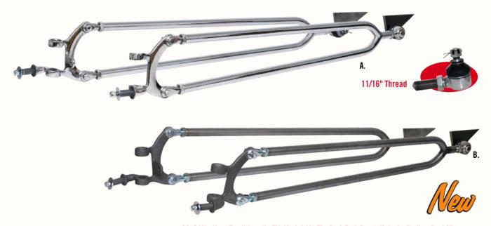
SO-CAL's New Traditionalist<sup>TM</sup> Model 'A' Tie Rod End Front Hairpin Radius Rod Kit: This new Model 'A' hairpin radius rod kit includes our revolutionary S/S batwing with integral lower shock mount, S/S clevises, S/S tie rod ends, frame mounting brackets and steel hairpins. They are available in plain or chrome hairpins with polished S/S components.
