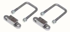
Model 'A' Rear Spring U-Bolt Kit: This kit is a direct replacement for '28 to '31 Model 'A' Ford stock rear crossmembers. It has a fabricated steel base plate, 9/16"-18 threaded mild steel U-bolts and Nylok nuts. #001-62175 Model 'A' rear U-bolt kit: \$59.94 pr.
