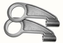
**Rear Buggy Spring Hangers:** These hangers are designed to be slipped over 3" dia. rear axle housing tubes then welded in place
