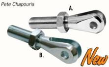
Rear Clevises: We offer two types of clevises for rear ladder bars; (A) polished S/S, 5/8"-18 male shank with a 7/16" hole and (B) zinc plated steel, 5/8"-18 male shank with a 7/16" hole. Both clevises have a 3/8" slot and jam nut. (A) #001-62128 Rear S/S clevis, 7/16" hole:
