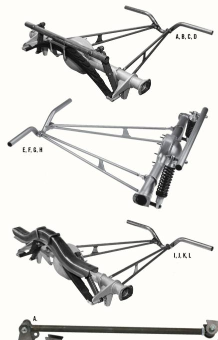
**9" Ford Rear Panhard Bar Kit:** Rear panhard bars are not only a must on coil-over but 'A'/40's style buggy spring rear suspensions as well. The kit stabilizes the inherent problem of lateral movement in early Ford type spring shackles and/or coil-over shocks. The adjustable bar measure 24 3/4" ( $\pm$  3/8") center to center, comes in plain steel or polished S/S and with or without frame tabs for those who already have a SO-CAL frame.
