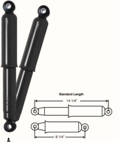
Covered Speedshocks in Steel: These nitrogen filled gas shocks are engineered specifically for hot rod applications and are offered in the "Standard" length of 9 1/4" closed and 14 1/4" extended. The distinctive design of the dustcover is reminiscent of the "airplane shocks" used on early hot rods during the 40's and 50's. Other features are 90 durometer replaceable 5/8" ID lower and 7/16" ID upper neoprene rubber bushings and they come finished in either high gloss SO-CAL red or show chrome.
