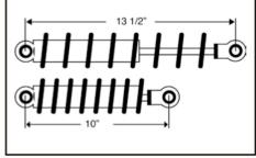
Coil Over Shock Bolt Kits: SO-CAL has developed these easy-to-install upper and lower coil-over shock bolt kits. Upper kit includes 6" Grade 5 bolts, full locking nut and optional crossmember tube. Lower kit includes tapered spacer.
