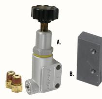
Proportioning Valve: Manufactured by Wilwood this proportioning valve lets you fine tune the front-to-rear braking balance by proportionately decreasing the rear (or in some cases the front) brake line pressure. Pressure adjustments range from 100-1,000 psi. (A) #024-260-2220 Proportioning valve: \$53.17 ea. (B) #001-62138 SO-CAL Proportioning valve mounting pad: \$7.80 ea.
