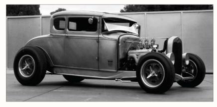
**Model A Headlights:** Shown above on Debra Kipps's SO-CAL-built A-V8 Coupe, these Model A headlights with fluted lenses offer yet another option for the traditional hot rod whatever the make, model and year.
