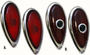
'39 Teardrop Taillights: With side-mounted bulbs in white powdercoated cast aluminum housings, these '39 teardrops are shallower than stock giving you more trunk space or apron clearance. Also, because the insides of the buckets are white, they're 30-percent brighter than stock lights.
