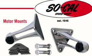
Small Block Chevy S/S Motor Mounts: Even though this pair of motor mounts is designed to accommodate a small block Chevy into a '32 and '33/"34 Ford chassis, we use them as universal mounts for almost anything including mid-50's shoe box cars. They are investment cast 17-4 S/S and come with trim-to-fit weld on frame mounting tabs.
