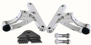
Ford Aluminum Motor Mounts: This pair of mounts accommodates both Windsor and Cleveland engines for '32 and '33/'34 Ford chassis. They are CNC machined from 6061 Aluminum alloy and come with trim-to-fit weld on frame mounting tabs. #001-62803 Motor mount Ford aluminum pol.: \$194.95 pr.
