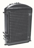
Walker Radiator: SO-CAL offers a full range of Walker radiators, however, two types of the popular Walker Cobra Z-Series radiator are perfect for all '32 Fords up to heavy-duty and big-block applications. The Cobra Z Cool-Mate Series includes an air-conditioning condenser. Call for applications and
