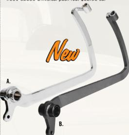
Brake Pedal, Automatic Transmission: This brake pedal offers the correct leverage for easy operation and is designed for the SO-CAL Step-Boxed™ frame but other applications apply. The threaded end accepts the stock Ford style pedal pad or any of the SO-CAL pads. Available in plain or show quality chrome.
